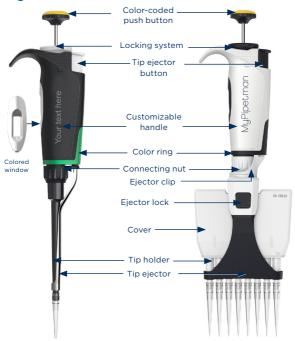
Figure 1 MYPIPETMAN® single channel and multichannel model components
